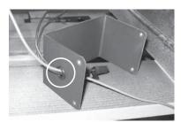
28) Attach the ground wire to the DC spark mounting bracket.
